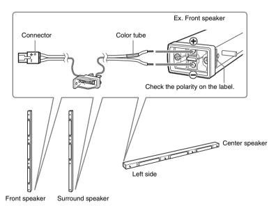
Insert the speaker cords into the speaker terminal of the speaker as far as they will go. Ensure that the cords are secure by gently pulling on them one at a time.
